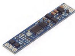
2-channel proximity dimmer. Four touch-free switching on, off and dimming of one channel. In Double White installations can change the colour temperature. Suitable for installation in aluminium profile. Detection range <18 cm (without diffuser).
